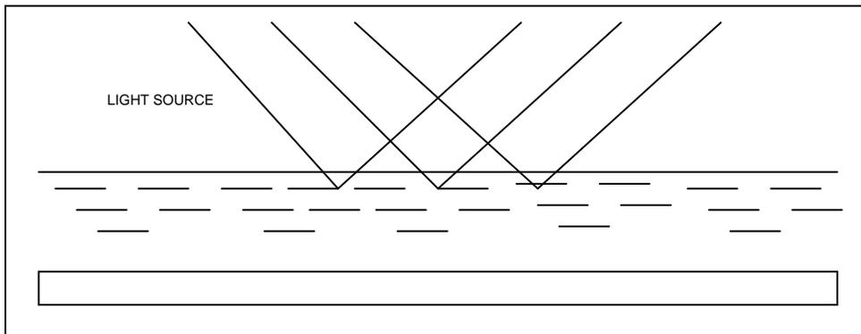
**Non-leafing** aluminum pigments generally use oleic acid, an unsaturated carboxylic acid, as the lubricant, and again this is absorbed onto the surface of the aluminum pigment. Oleic acid is compatible with powder coating polymer chemistries and, for this reason, the metallic pigment is oriented in a random manner throughout the bulk of the film. Very bright silver, chromatic silver and hammer finishes are achieved using non-leafing grade pigments.
