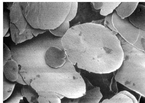
In the co-extrusion process, the aluminum pigment becomes completely encapsulated by the powder coating polymer. This results in powder coatings which:
