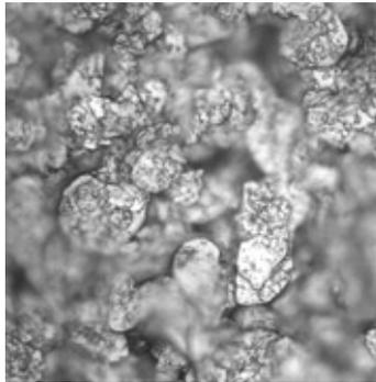
Aluminum metal is amphoteric, reacting with both acidic and alkaline environments. Under certain circumstances, this metal flake can react with acidic or basic systems, potentially resulting in less-than-desirable performance. Aluminum metal also has the capability of reacting with water, which is not a serious concern when dealing with large, fabricated pieces. In this instance a slow reaction occurs with the generation of a thicker, benign oxide or hydroxide layer. This
